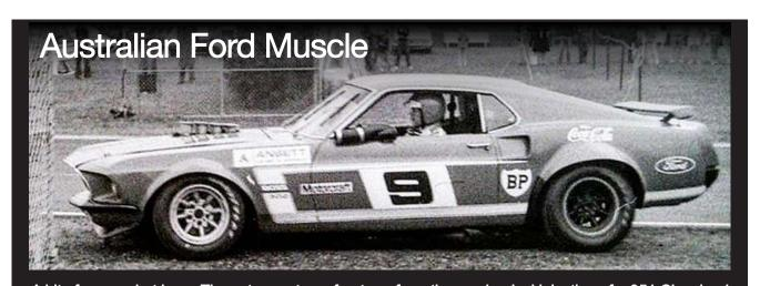
A bit of a rare shot here. Those trumpets up front are from the mechanical injection of a 351 Cleveland from Moffat's Super Falcon. Installed for some more straight line grunt, it upset the Car's fine balance and was removed shortly after. This photo is allegedly from the 1972 Sandown 250 support race, there's not too many shots of this legendary Car in this configuration.
