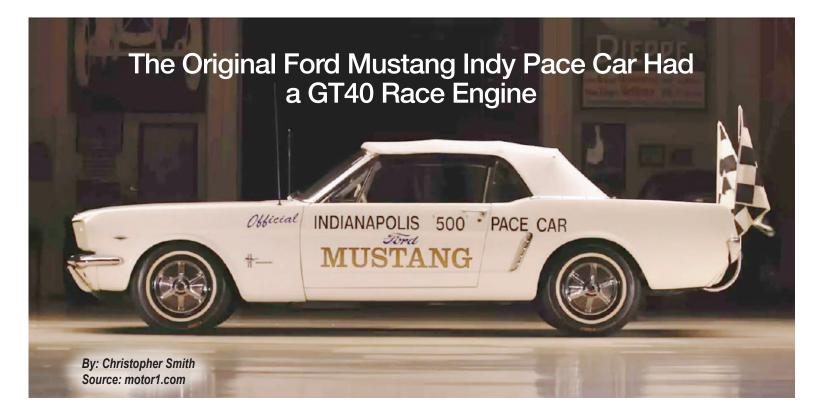
It wasn't fast enough to pace the field with the stock V-8, so it got a major bump in power. To meet the speed requirements for a pace car, it was fitted with a detuned engine from the Mark I Ford GT40 race car.
